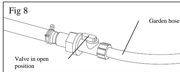
4. Route the garden hose to a sewer drain capable of safely assimilating 1135 liters (300 plus gallons) of water which may contain both unsanitary contaminants and chemical residue. Open the drain valve (as shown in Fig 8). The spa drains slowly.
